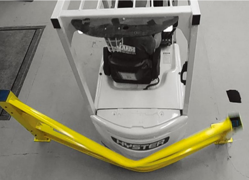
TRADITIONAL metal protection systems fails on impact.
